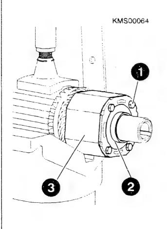
STARTING-MOTOR DISASSEMBLY Disassembling multi-plate clutch Full complete multi-plate clutch out of clutch housing.
